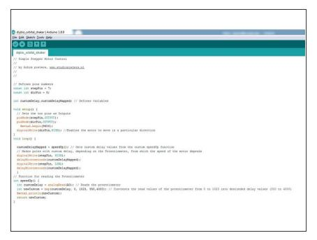
Program the Sparkfun Pro Micro via the Arduino IDE using the DIYbio orbital shaker firmware. Additional instructions regarding Arduino IDE settings for this microcontroller can be found here:
