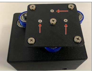
Use 3 tapered M3 x 12 screws to attach the labware adapter plate onto the bearing linkage.
